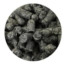
Stabilization and reinforcement of asphalt mixtures
